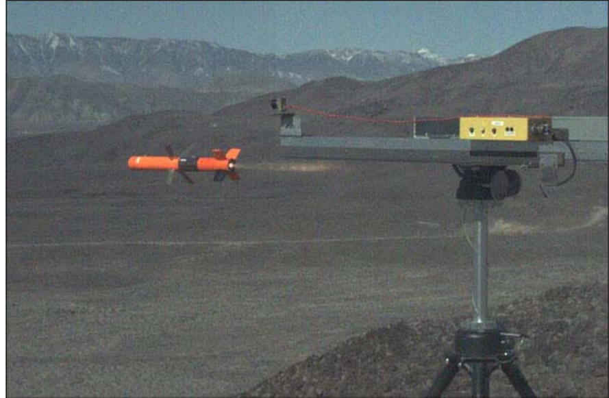
A Spike test missile is fired from the top of a small mountain on the China Lake range to simulate being launched from an unmanned air vehicle.
